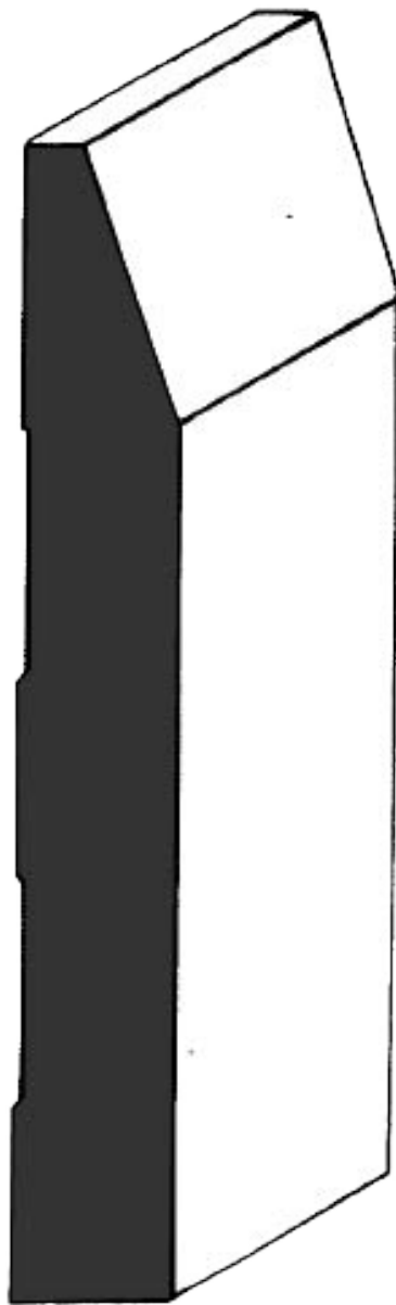
703-5 * This profile is available in multiple height options. 5/6" x 5 1/2"
