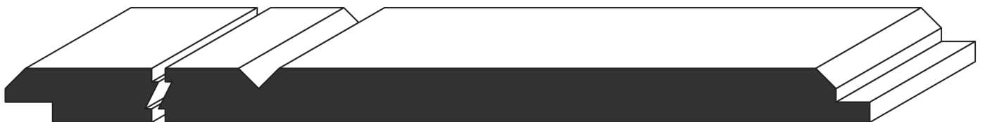
MDF 1248-ITC-VG-514 1/2" x 4' x 8' vee grooved, approx. 5 1/4" OC
